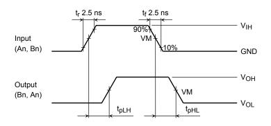
Figure 2 t<sub>pLH</sub>, t<sub>pHL</sub>
